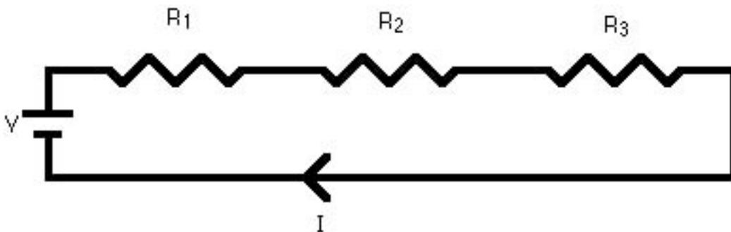
A series circuit is shown in the diagram above. The current flows through each resistor in turn. If the values of the three resistors are:
