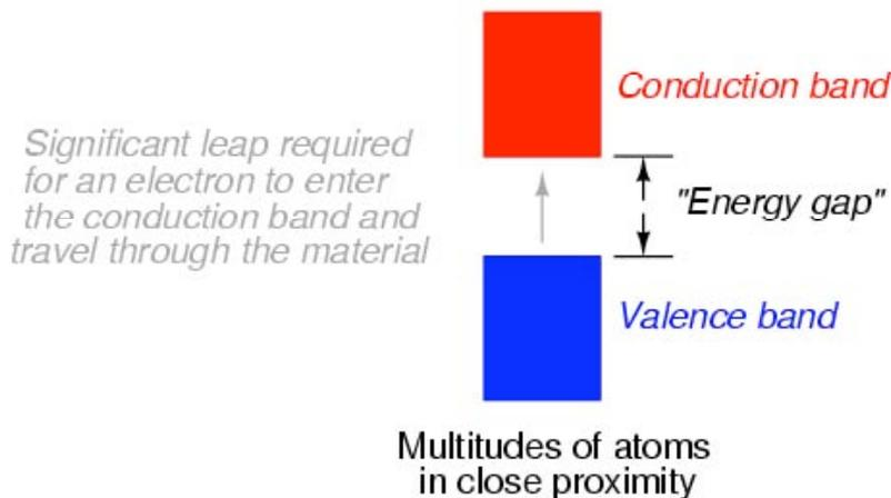
Materials that fall within the category of semiconductors have a narrow gap between the valence and conduction bands. Thus, the amount of energy required to motivate a valence electron into the conduction band where it becomes mobile is quite modest:
