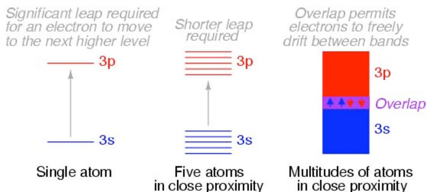
When atoms combine to form substances, the outermost shells, sub shells, and orbitales merge, providing a greater number of available energy levels for electrons to assume. When large numbers of atoms exist in close proximity to each other, these available energy levels form a nearly continuous band wherein electrons may transition.
