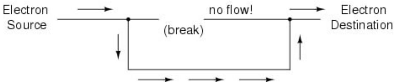
Now, we have continuity from the Source, to the newly made connection, down, to the right, and up to the Destination. This is analogous to putting a "tee" fitting in one of the capped-off pipes and directing water through a new segment of pipe to its destination. Please take note that the broken segment of wire on the right hand side has no electrons flowing through it, because it is no longer part of a complete path from Source to Destination.
