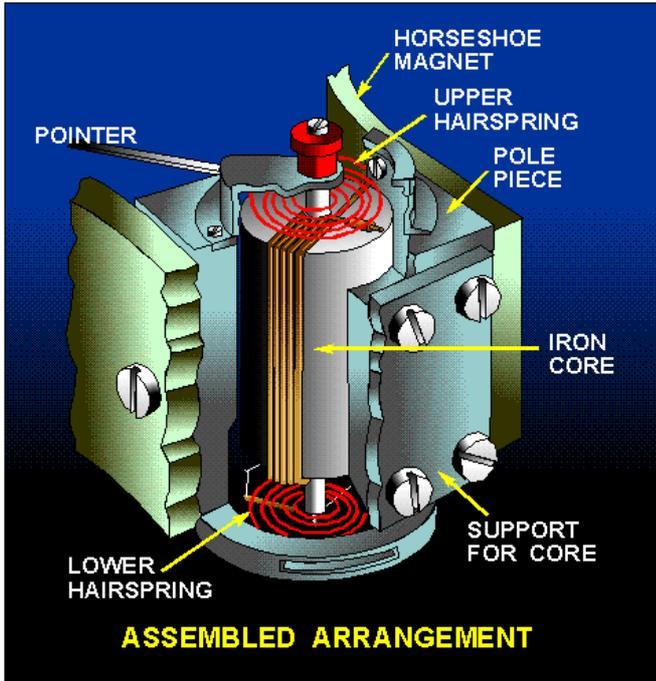
**Figure 1.** This permanent-magnet moving-coil meter movement is the basic movement in most measuring instruments. It is commonly called the d'Arsonval movement because it was first employed by the Frenchman d'Arsonval in making electrical measurements. Figure 1-10 is a view of the d'Arsonval meter movement used in a meter.
