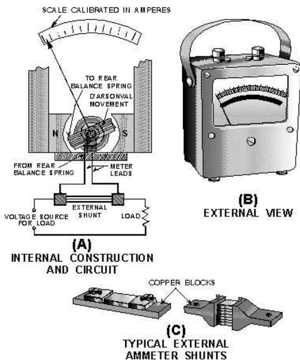
For higher current ranges (above 50 amperes) ammeters that use external shunts are used. The external shunt resistor serves the same purpose as the internal shunt resistor.
