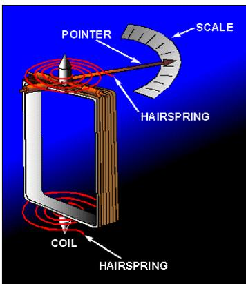
**Figure 3.** With the use of hairsprings, the coil will return to its initial position when there is no current. The springs will also tend to resist the movement of the coil when there is current through the coil. When the attraction between the magnetic fields (from the permanent magnet and the coil) is exactly equal to the force of the hairsprings, the coil will stop moving toward the magnet.
