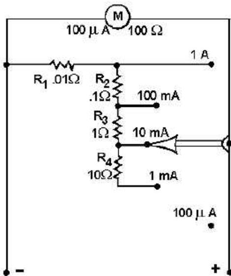
Most meter movements in use today have sensitivities of from 5 microamperes to 1 milliampere. **Figure 7** shows the circuit of meter switching to different ranges.
