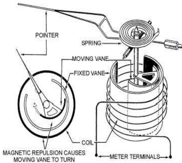
**Figure 4.** The moving-vane meter operates on the principle of magnetic repulsion between like poles.
