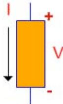
The voltage across the device is a measure of the energy - in joules - that a unit charge - one coulomb - will dissipate when it flows through the device. If the device is a resistor, then the energy will appear as heat energy in the resistor. If the device is a battery, then the energy will be stored in the battery.
