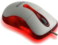
The optical mouse was an advancement of the Trackball in that it used an optical sensor to detect movement. An LED would shine onto the surface underneath the mouse and this allowed a sensor to detect the detailed surface.
